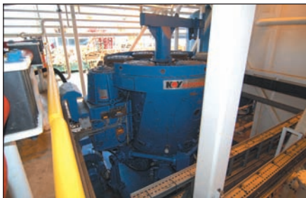
Prototype NOV Hex fluid pumps after one year of service.
