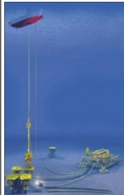
How Well Enhancer's riserless intervention system will be deployed onto a subsea tree.
